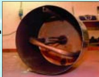
The QL Water Heater has a tank capacity of 20 litres and can be mounted horizontally and vertically. The water heater has simple feet that are spot-welded to a strap that goes round the tank.
