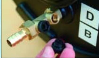
**DRAIN:** The tank of the Vetus is drained by unscrewing a plastic lid. This solution will result in waste-water when the tank has to be drained.
