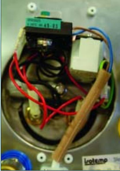
**SAFETY THERMOSTAT:** The Isotemp is the only water heater in the test with a safety thermostat that works on boiling dry. The blue "box" is the safety thermostat, while the operating thermostat is the white "box".
