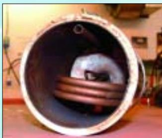
← THE HEATING COIL is strong and well dimensioned. The water heater ought to have had rather better insulation.
