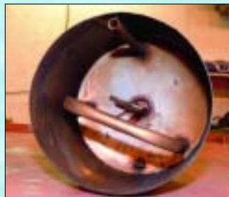
The Mobitherm has a capacity of 20 litres, and can be mounted horizontally and vertically. The water heater has simple feet spot-welded to a strap that goes round the tank. Both the tank and heat exchanger are made of high-quality acid-proof steel (AISI 316). The insulation is of polyurethane foam, but is not equipped with any protective casing.
